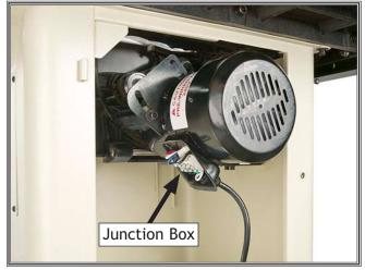
Figure 111. Motor junction box location.
